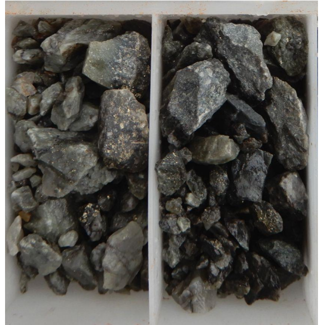
Plate 1. RHRC0022 with sulphide mineralisation 2m @ 29.16 g/t Au from 121m (incl. 1m @ 43.34g/t Au)
