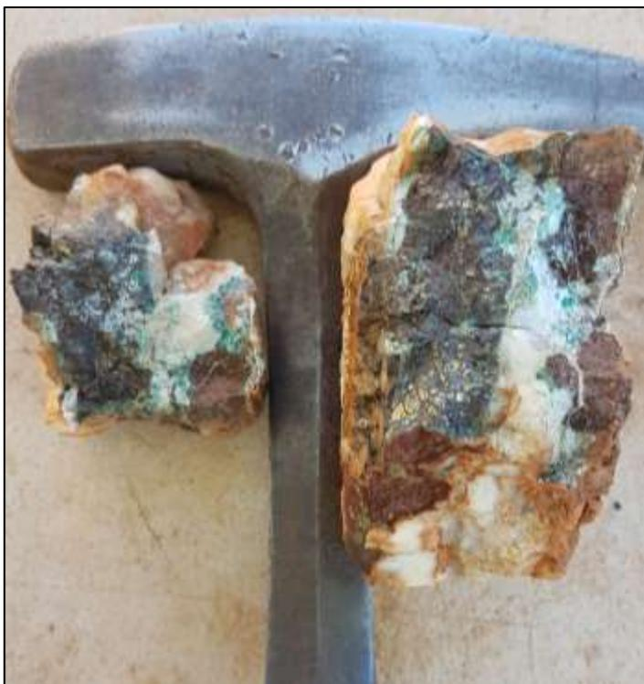
Figure 2: Rock chips samples of the high copper-gold vein in the older Archaean basement.
