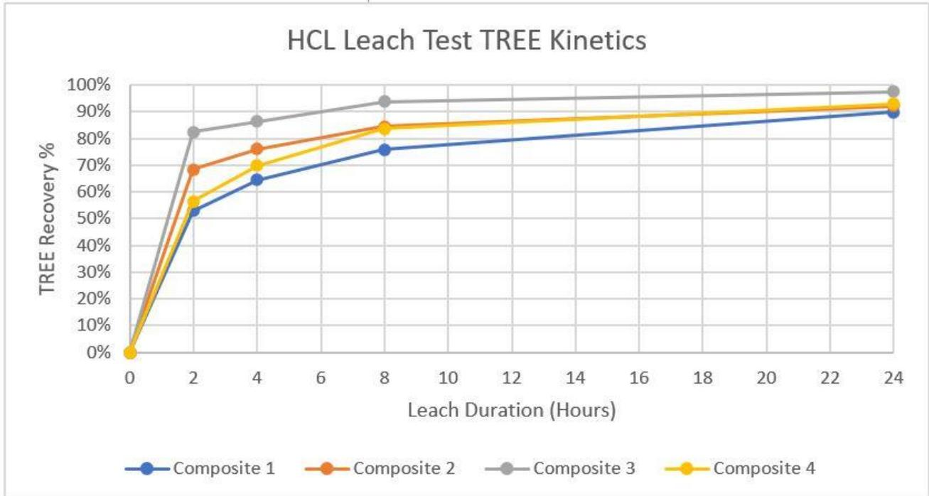
**Figure 7.** Chart showing leach test results for four composite samples from Black Cat in HCl at 25g/L concentration and 50°C temperature over 2, 4, 8 and 24 hours.
