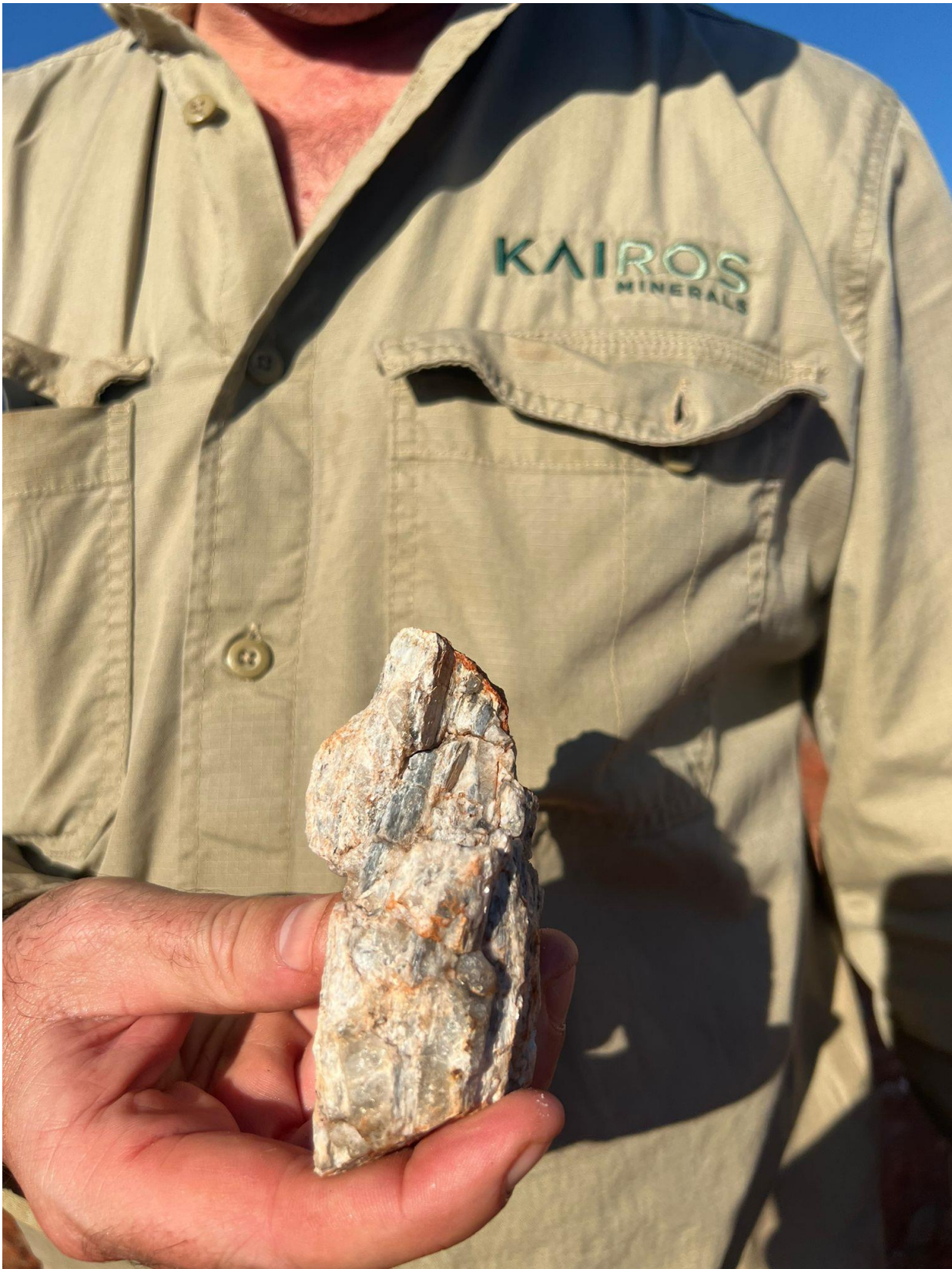
Figure 1. Kairos Geologist Campbell Watts holding a piece of spodumene-bearing pegmatite (MYR393 - 1.91% \text{Li}_2\text{O} ) discovered at 'Lucky Sump' during routine earth moving activities.
