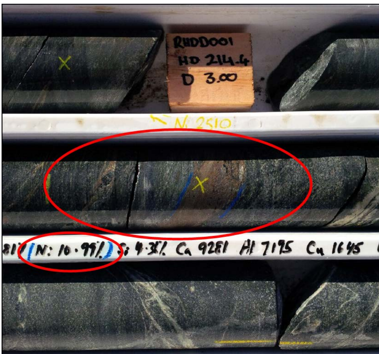
Figure 1: Drill core photograph showing the high grade Ni-Cu sulphides in the mineralised vein within ultramafic rocks. Note Ni grades from field PXRF analysis.
