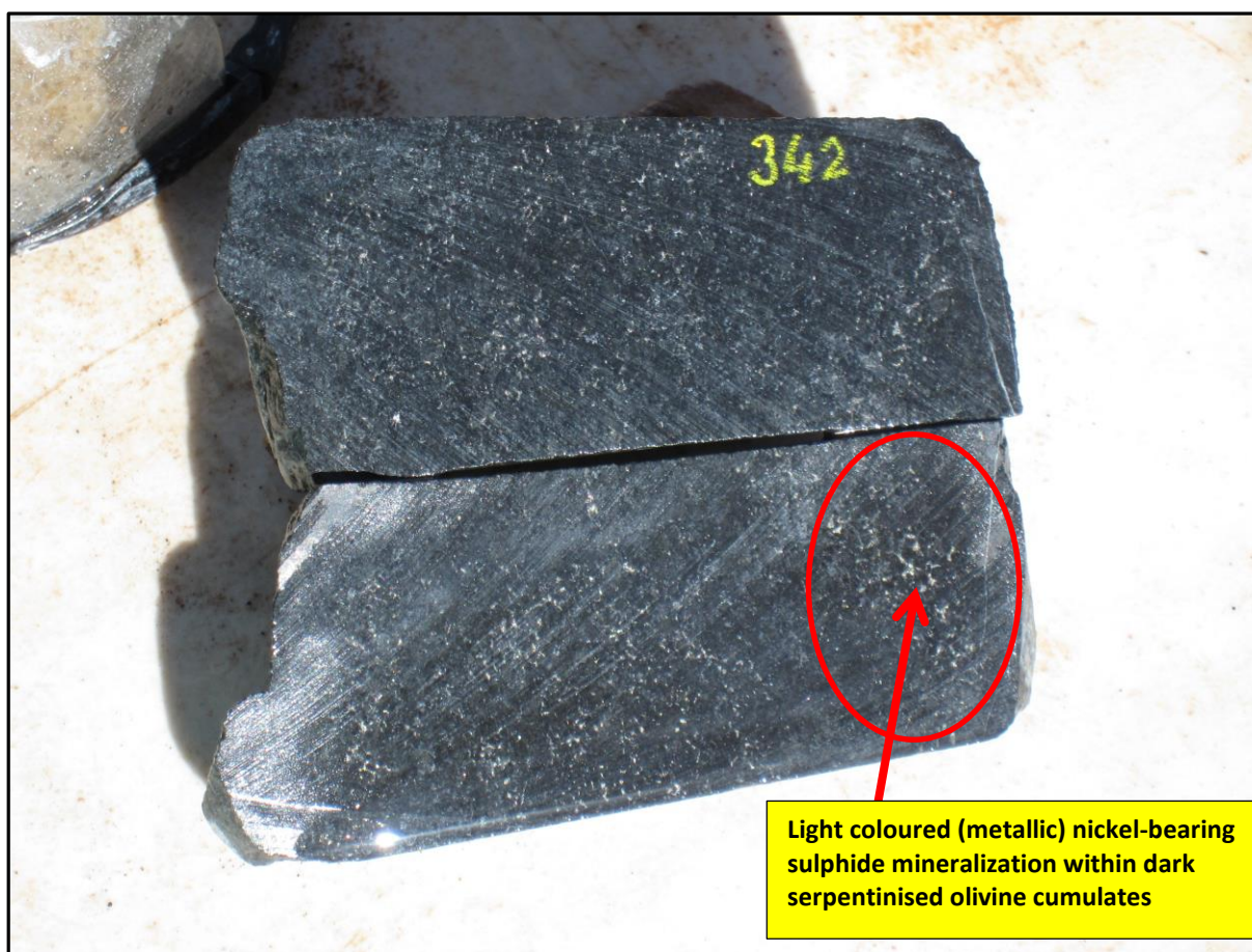
Figure 1: Strongly disseminated nickel sulphide mineralisation at a depth of 342m within RHDD0012 drill hole at Roe 1 Prospect. The mineralisation is hosted within a serpentinised meso-accumulate ultramafic.
