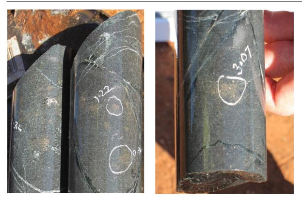
Photo's 2 and 3: Disseminated and Blebby Nickel Sulphides hole RHDD0015
