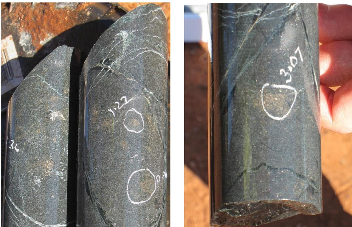
**Photo's 2 and 3: Disseminated and Blebby Nickel Sulphides hole RHDD0015**
