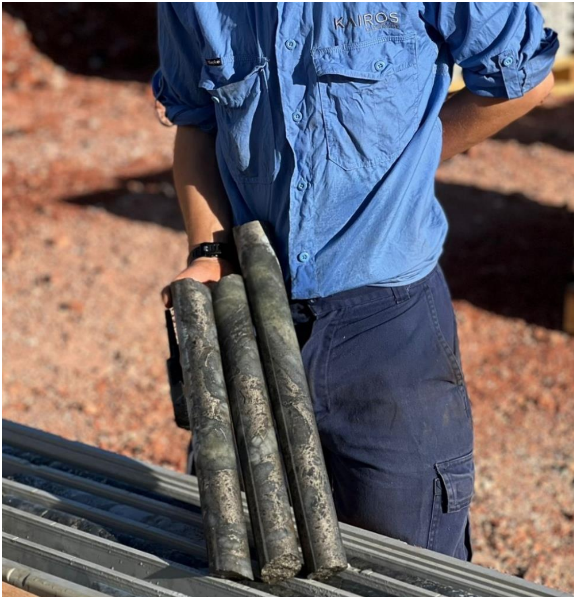
Figure 6 - Kairos geologist Will Coussens with core from hole KMYD071 showing extremely silicified and sulphidised (pyrrhotite, pyrite, arsenopyrite, chalcopyrite) wall rocks at the hangingwall contact of a well mineralised banded iron formation. The mineralisation is typical of the hangingwall sequence and is 15.4m in down-hole thickness at this location at Main Hill prospect (see Figure 8).
