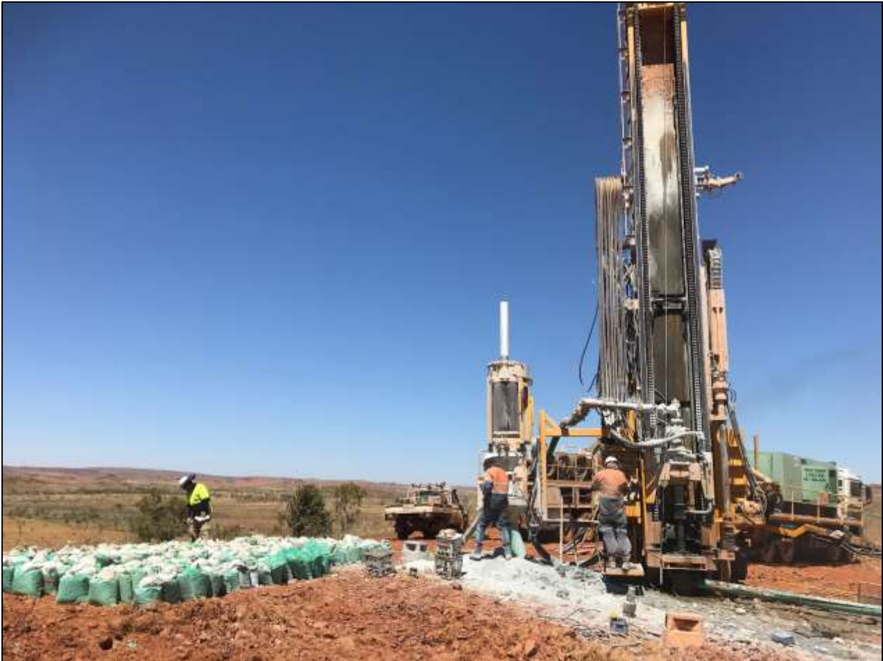
Figure 3: Mt Magnet Reverse Circulation (RC) drill rig operating at the Fuego prospect, Croydon Project.
