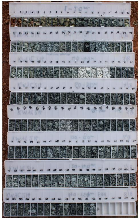
**Figure 3.** RC chips for hole KMYC216 drilled directly underneath Lucky Sump where surface spodumene-bearing pegmatite samples returned up to 1.91% Li₂O. Note the white chips in metres 52-56m. Results pending.
