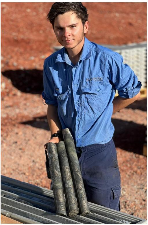
**Figure 4.** Kairos geologist Will Coussens with core from hole **KMYD071** showing extremely silificied and sulphidised (pyrrhotite, pyrite, arsenopyrite) wall rocks at the hangingwall contact of a well mineralised banded iron formation. The mineralisation is typical of the hangingwall sequence and is **15.4m** in down-hole thickness at this location at Main Hill prospect (see **Figure 5**).
