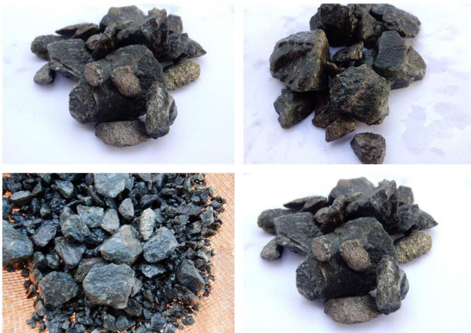
Plate 1. Sulphidic dolerite identified in rock chips – RHRC009 ~94m downhole.
