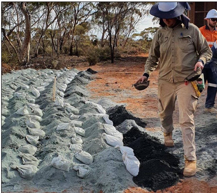
Figure 1: Significant zone of sulphides (darker samples) intersected in hole RHRC120 at Black Cat Prospect.
